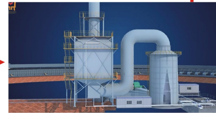
Smoke Cleaning and Desulfur Tower
