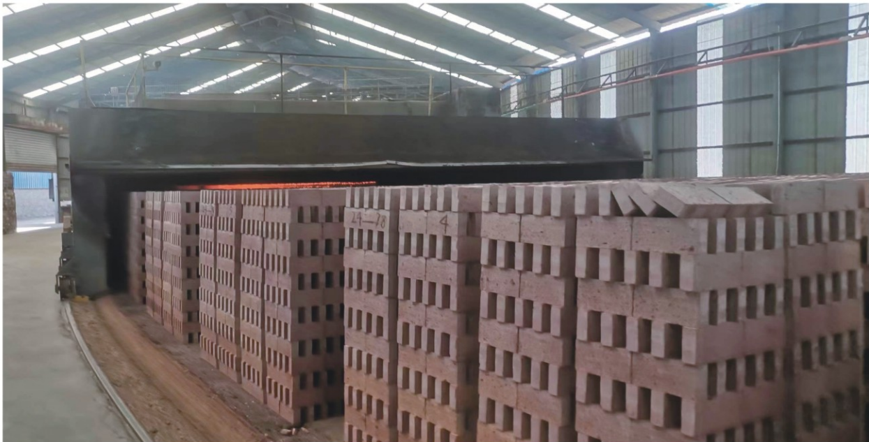
Project Name: Mongolia Jia He Tian Hua Co., Ltd Location: Ansu town, Etoke Front Banner, Erdos City, Inner Mongolia Kiln Section: 11.2m Kiln Capacity: 300000 bricks/day Raw Materials: Water-based cuttings
