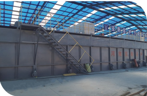
Project: Aksu Dingsheng New Building Materials Co., Ltd Location: Aksu, Xinjiang Kiln Section: 12.98m Kiln Capacity: 400000-500000 bricks /day Materials: shale, coal gangue, construction waste
