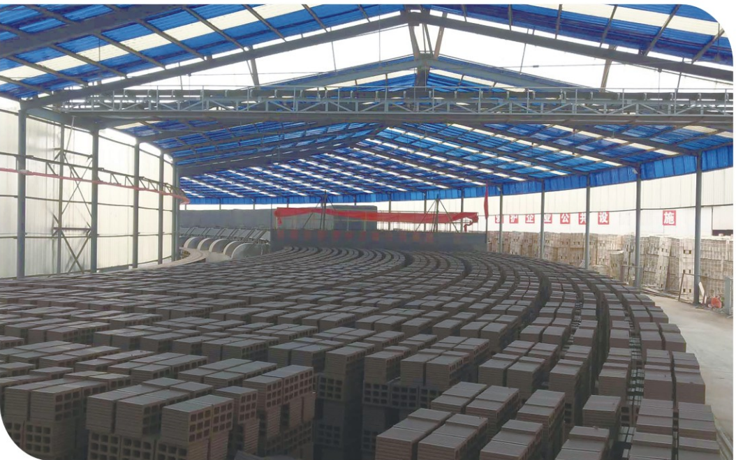
Project: Aksu Dingsheng New Building Materials Co., Ltd Location: Aksu, Xinjiang Kiln Section: 12.98m Kiln Capacity: 400000-500000 bricks /day Materials: shale, coal gangue, construction waste
