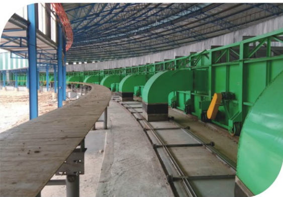
Project: Quang Binh, Brick Factory Location: Quang Binh, Vietnam Kiln Section: 11.8m Kiln Capacity: 400000-500000 bricks /day Materials: shale, river sludge, construction waste, industrial tailings
